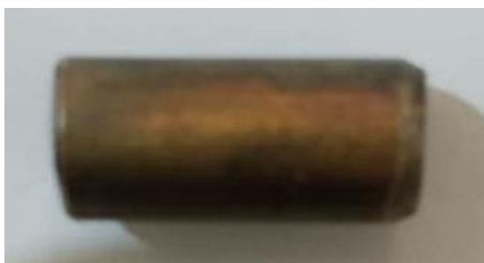
Fig. 4: Specimen after the immersion in Gabraun water without inhibitor
