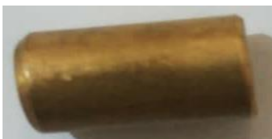
Fig. 3: Specimen after the immersion in Gabraun water with inhibitor
